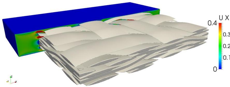
**Figure 2:** Viscosity field  $U_x$  of three layered triaxial 12k braid (RVE)
