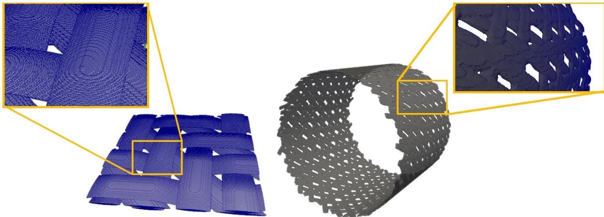
**Figure 1:** *One layer triaxial 12k braid RVE model (left), 3D near-net-shape triaxial 12k braid model (right)*
